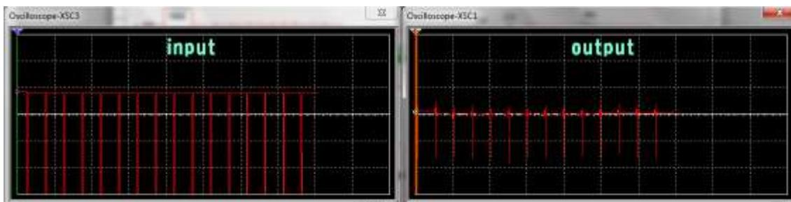
Figure 11. PWM transmitted signal (left) and the received signals (right)
