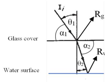
Figure (3) incidence, reflection and refraction angles of solar radiation
