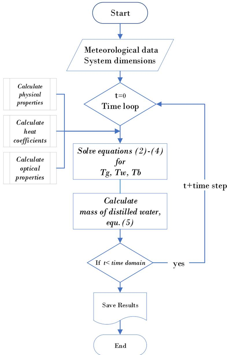
Figure (4) flowchart diagram for the present simulation model
