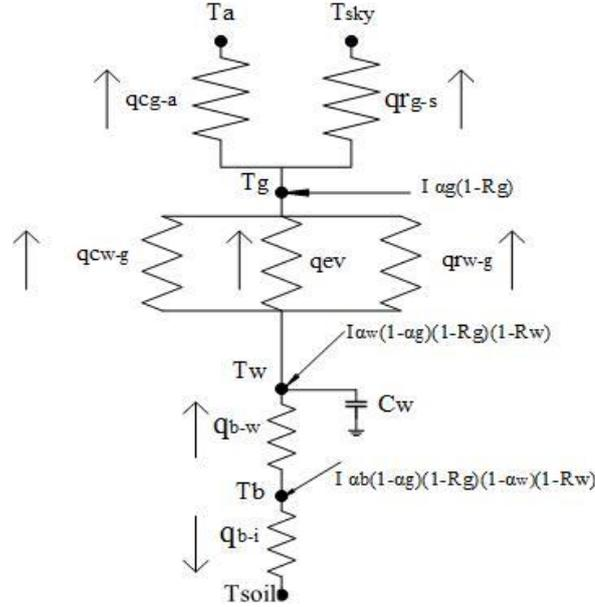
Figure (2) thermal network of present model
