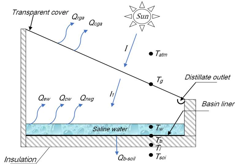
Figure (1) Thermal distribution of Solar desalination system
